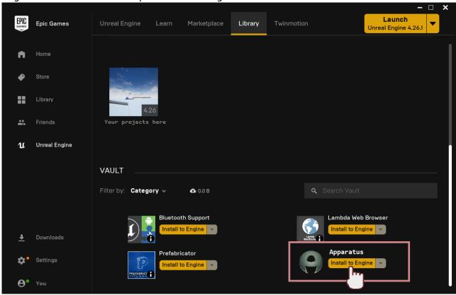
In the opened section choose the version of Unreal Engine. Note that you should use 4.26.1 (or above) as it's the only officially supported for now. After clicking 'Install' wait for a minute while the launcher loads the necessary files to the engine. When the installation has completed, you can verify its success by clicking the 'Installed Plugins' footer under Unreal Engine version you have installed the plugin for. 2025/11/02 22:37 2/13 Apparatus: Beginner's Guide
